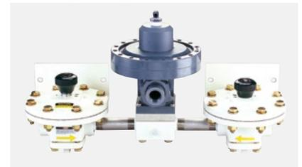
vacuum overcomes the latching force of the detent and the standby supply comes online along with the original supply. Automatic switchover valves are available only with capacities to 60 kg/h (3,000 ppd) of chlorine and are not for use with evaporators. A liquid-chlorine switchover system is available for evaporators.
