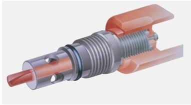
The V-notch orifice consists of a precisely grooved plug sliding in a fitted ring. Any position of the plug in the ring results in a specific orifice size
