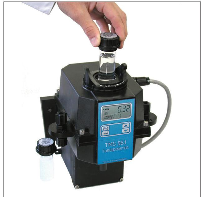
TMS 561 turbidimeter with Calibration Cuvettes
